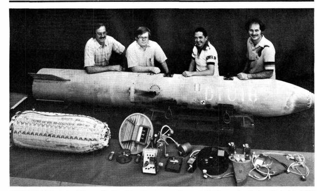
COMPONENTS of the B83 are displayed by these men who work in the mechanical and electrical B83 project divisions. Included are the packed parachute (at left), aft filter pack, preflight controller, firing set, and drop test unit itself. From left, Mike Neuman, Rex Eastin (both 8153), Rodger Page and Jim Dremalas (both 8152).
